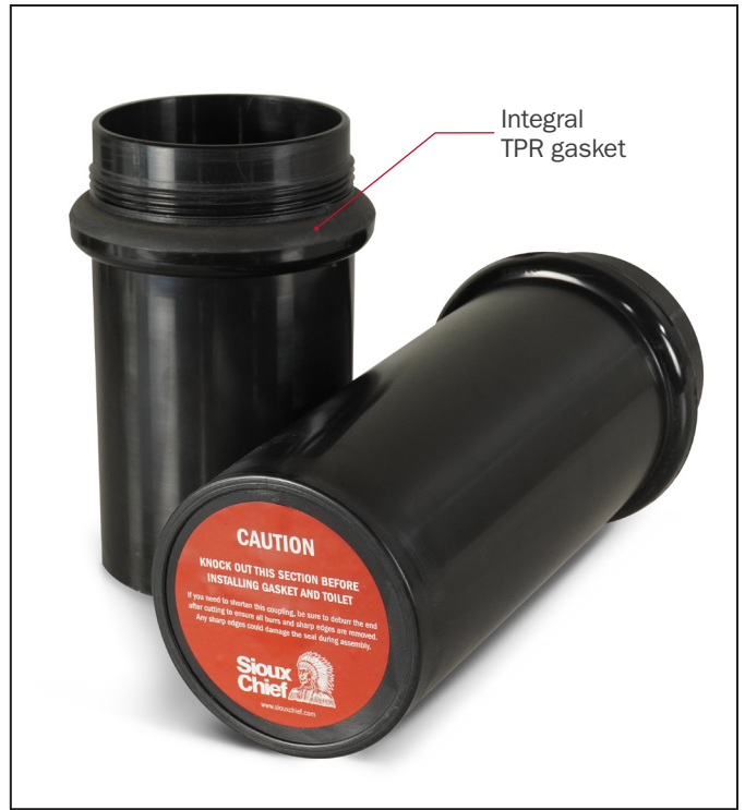
Newly-designed ABS couplings include knockout test cap and integrally-molded, TPR gasket, which seals tight with corresponding taper on faceplate.
